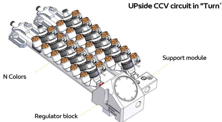
The performances are identical to the "In line" assembly having the same number of colors, it allows to optimize the dimensions in the arm of the robot.
