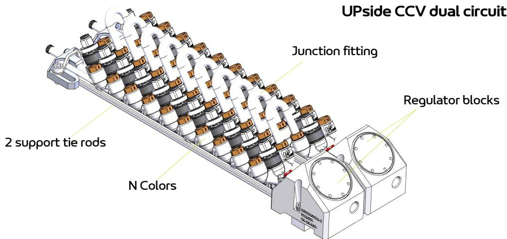
Used with the dual circuit atomizers, it makes it possible to work in masked time. Only one paint supply is necessary for 2 independent paint antennas. It is recommended for installations with 12 colors maximum.
