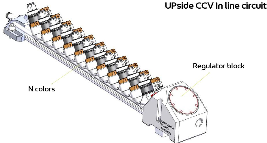
**Remarks:** Standard assembly, the "In line" circuit is used for installations going up to twelve colours. It is possible to go up to 24 colours subject to compatibility with the cycle times of the installation.
