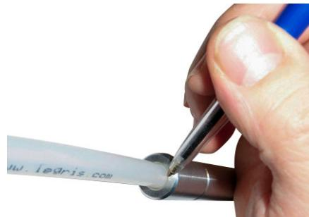
Coat with white assembly paste PTFE (P/N # F6RXZZ129) the hose on a 1 cm length. It is imperative not to cover the mark.
