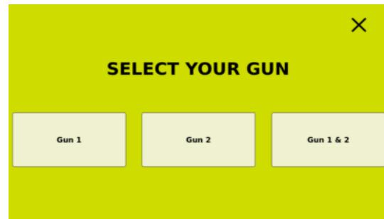
Following the selection of the recipe in the case of a configuration with only one gun or following the selection of the gun(s) in the case of a configuration with two guns, the Cyclomix® Evo automatically switches to the priming phase
