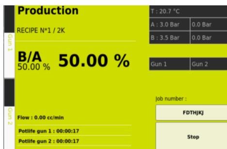
Activation is either via the button on the main or remote display, or via a 24V signal connected to input N°6 for gun 1 and N°7 for gun 2 on the DIOB 1 board in the main cabinet.
