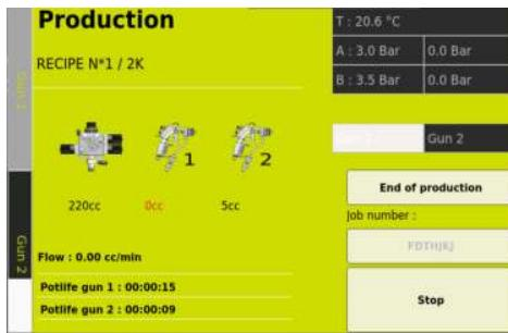
Then the volume of each circuit will decrease according to the use of the gun (gun open information thanks to the air atomization flow control).
